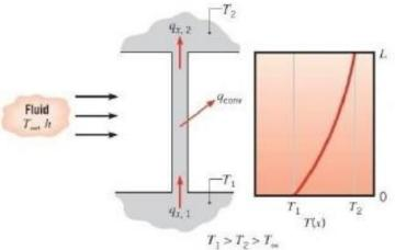
strut is used to provide mechanical support to two walls at different T. A temperature gradient in the x-direction sustains heat transfer by conduction internally, at the same time there is energy transfer by convection from the surface.
